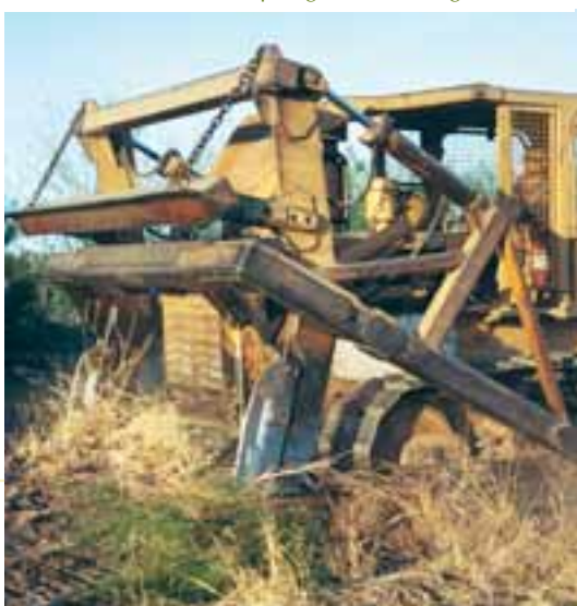
▼ Front-mounted blade plough (Ellrott design)
